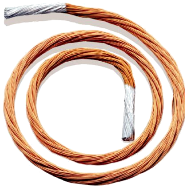
Litz Wire Size: 0.125mm Configuration: 5x3x28
